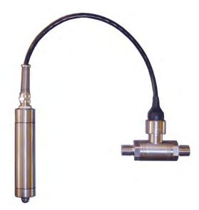
The internal temperature sensor provides accurate temperature measurements without the need for a separate temperature recorder. The logger can be started to take measurements as often as every two seconds, up to one reading every twelve hours. It will store up to 16,383 readings in its non-volatile memory.
