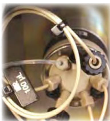
Exchangeable Sample Loop made of PEEK
