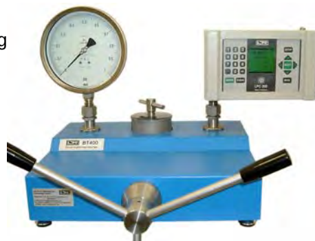
BT400-OX with Calibrator LPC 300 and test item
