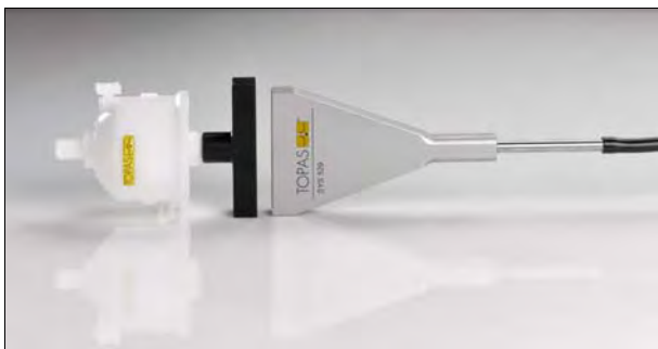
Isokinetic rectangular sampling probe for a volume flow rate of 28.3 l/min (1cf/min) at 0.45 m/s air velocity and adapter piece with HEPA filter for cleaning purposes
