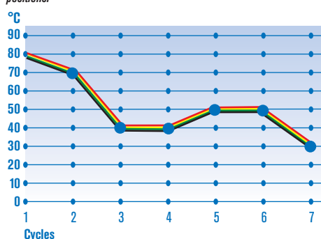
Graphic detail that shows temperature perfect uniformity in the different block wells, distinguished by different colours: red, yellow, green, black. It also shows how uniformity is maintained during all the thermal cycle periods, previously programmed in the display.
