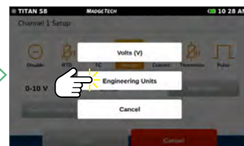
Select Engineering Units
